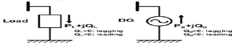
Fig3: Load models and DG as their power factor
