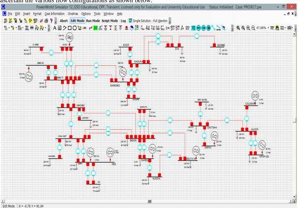
Figure 4: Existing 330KV transmission network with scheduled load in the PWS Edit mode
