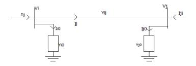
Figure 2: Transmission line model for calculating line flows.
