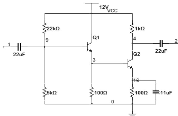
**Figure 1:** Schematic diagram of the conventional Darlington pair amplifier
