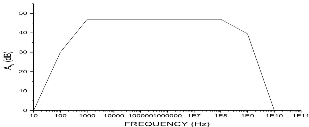
**Figure 4:** Frequency Response of the Distributed Amplifier (Simulation)
