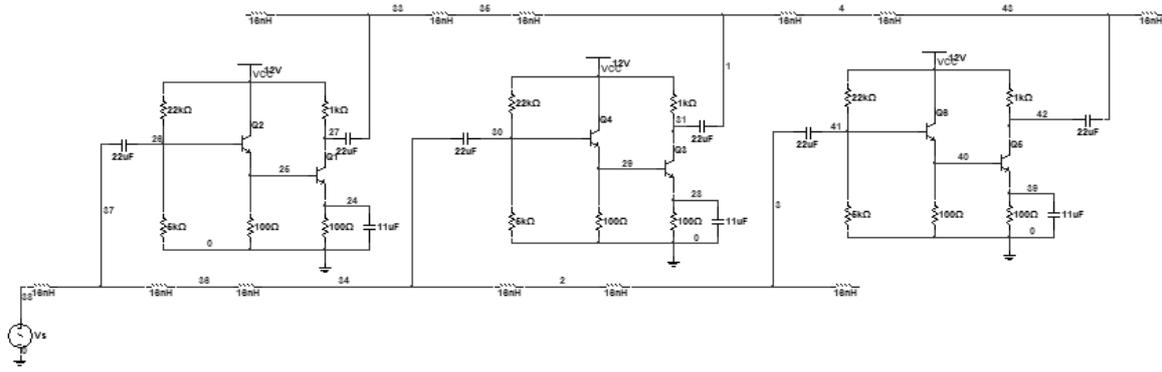
Figure 2: Schematic diagram of the distributed amplifier.
