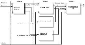
Fig 2.Pipelined Floating point multiplier
