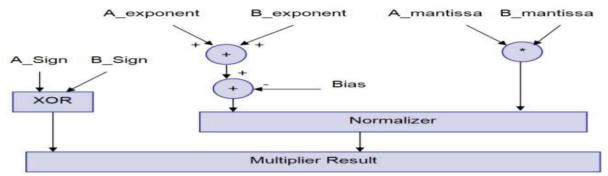
Fig. 1: Architecture for Floating point multiplier.
