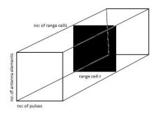
Figure 1: Radar Data Cube
