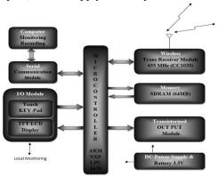
Fig. 3. Block Diagram for Central Monitoring Smart Node
