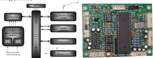
Fig. 2. Schematic Block Diagram for Remote Monitoring Smart Node&Slave Node HW (PIC 16F877) 2.3 Central Monitoring Smart Node (Master Unit)
