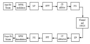
Figure 1: Block diagram of a baseband OFDM System
