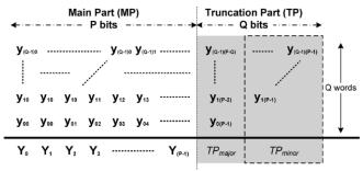
Fig:1: Q,P bit words shifting and addition operations in parallel.
