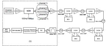
Fig.2. Experimental configuration of our proposed full-duplex ROF transport systems.
