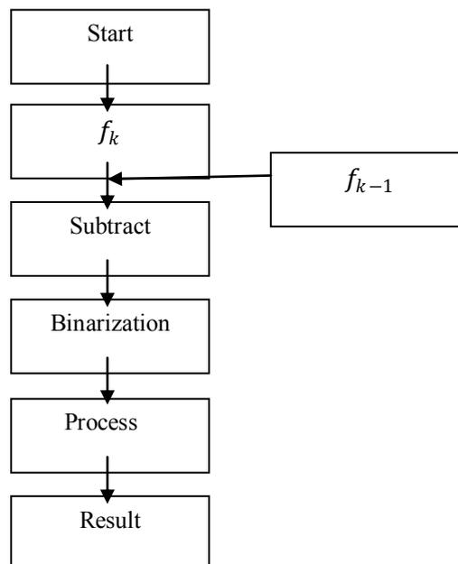
Fig.4. Flow chart for frame difference method
