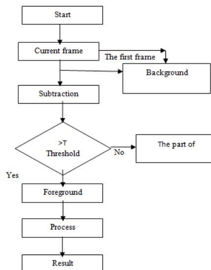
Fig.1. Flow Chart for background subtraction algorithm
