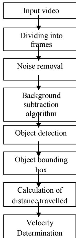
Fig.5. Flow chart of object velocity determination
