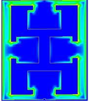
Fig-(3.11) current distribution of final patch shape
