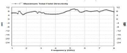
(Fig-(3.10): directivity Vs Frequency graph 1<sup>st</sup> iteration)
