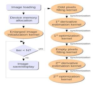
Fig.8. Flow chart representing the execution of the CUDA ICBI implementation. Ellipses represent kernels where matrices are processed in parallel creating multiple threads each one processing a separate block.
