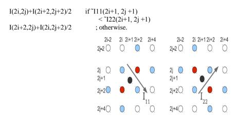
Fig. 2. At each step (here it is shown the first), the FCBI algorithm fills the central pixel (black) with the average of the two neighbors in the direction of lowest second order derivative (II1 or I22). II1 and I22 are estimated using for each one the 8 valued neighboring pixels (evidentiated with different colors).
