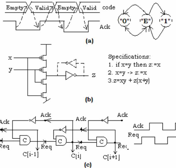
Figure 2. (a) The 4-phase dual rail logic (b) Muller C-element and indication concept and (c) Muller Pipeline
