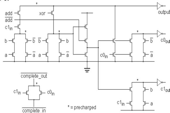
Figure 3. The Adder Circuit in ALU
