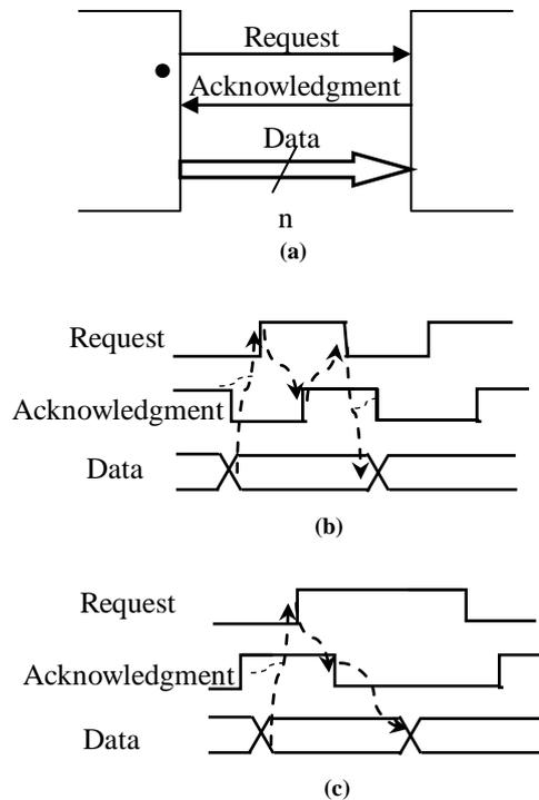
Figure 1. (a) A bundled-data channel (b) A 4-phase bundled-data protocol (c) A 2-phase bundled-data protocol
