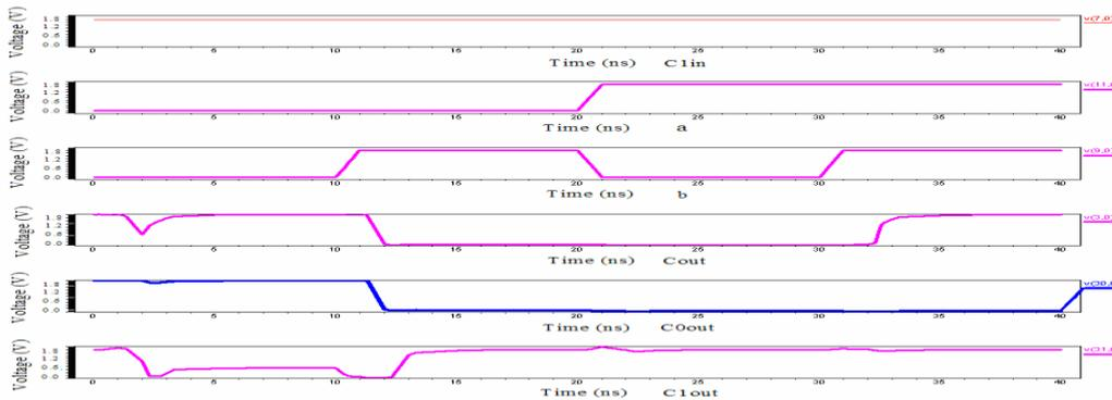
Figure 5. Simulated waveforms for the 1 bit addition operation
