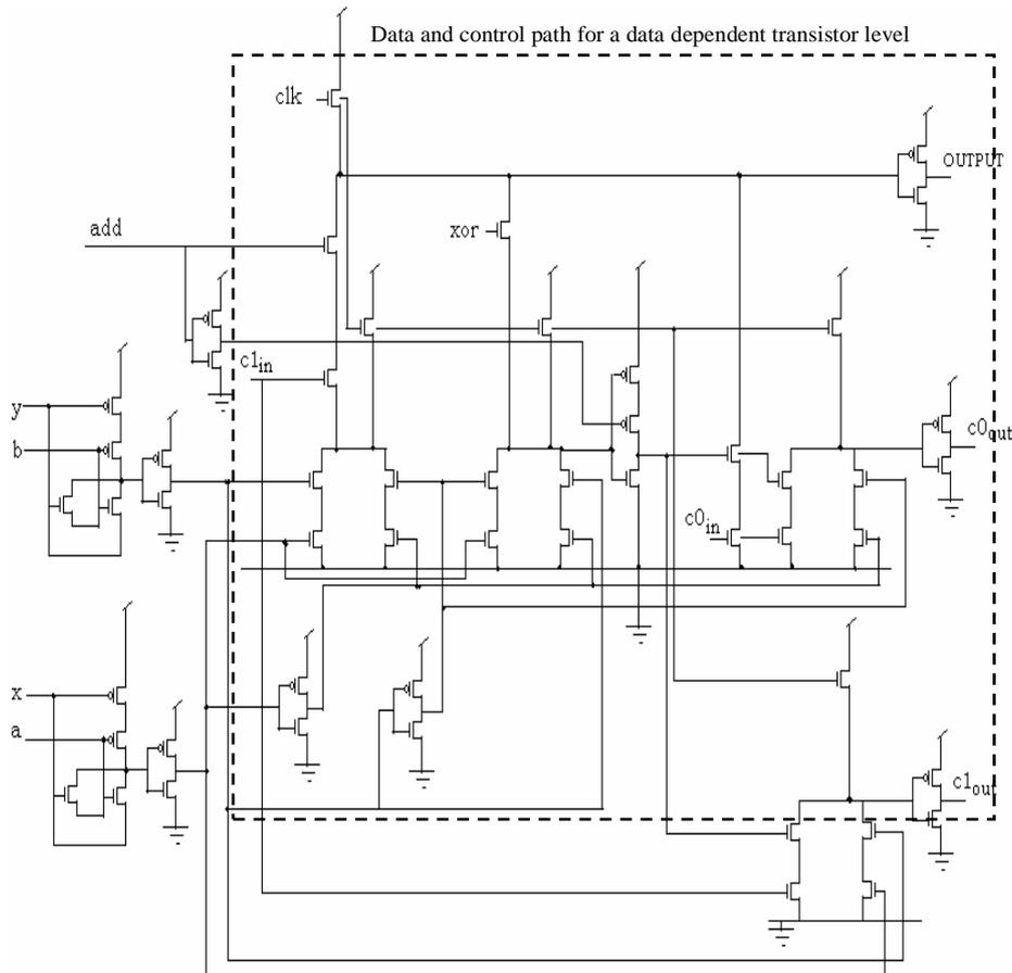
Figure 4. A CMOS level Asynchronous ALU circuit for 1-bit operation
