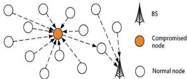
Fig. 6. Sink Hole Attack
