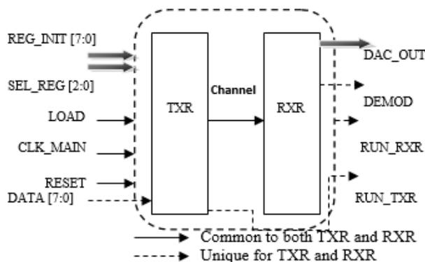
Fig. 3. Block Diagram of MC-CDMA with Transmitter And Receiver
