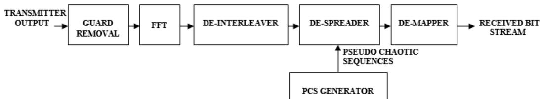
Fig. 5. Block Diagram of MC-CDMA Receiver Using PCS Generator
