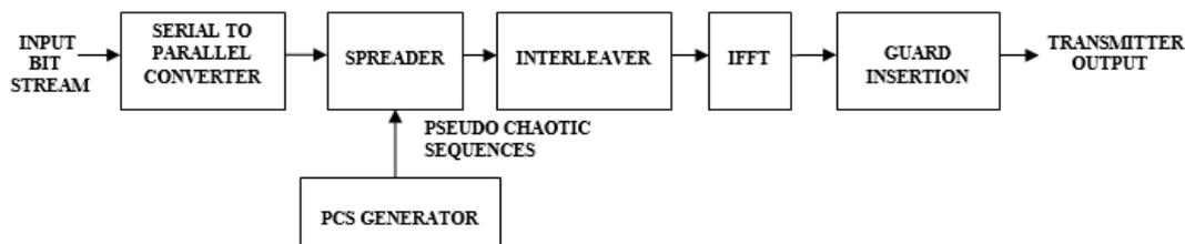
Fig. 4. Block Diagram of MC-CDMA Transmitter Using PCS Generator
