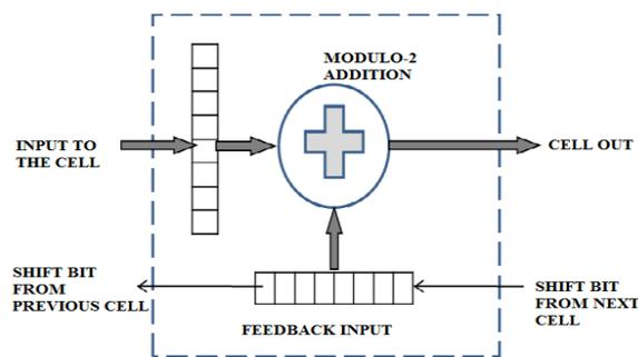
Fig. 1. Basic NLFSR cell structure
