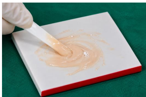
Figure 5 : Mixing nano-HA with Resin cement
