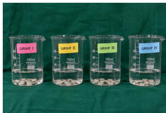
Figure 8 : Water solubility & sorption testing
