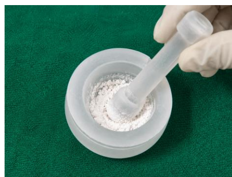
Figure 4: Mixing nano-HA with GIC
