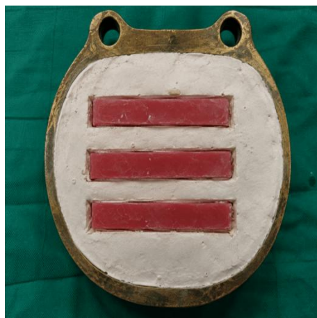
Figure 5: Wax blanks invested in flask for packing of heat cure
