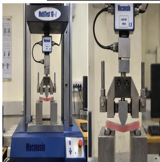
Figure 8: Flexural strength testing on Universal testing machine
