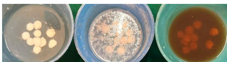
Fig 5: Immersion of TiO 2 incorporated Soft Liner in Distilled Water, Tea Tree Oil and Guava Leaf Extract
