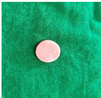
Fig 3: Soft liner samples incorporated with TiO 2 and 10mm diameter
