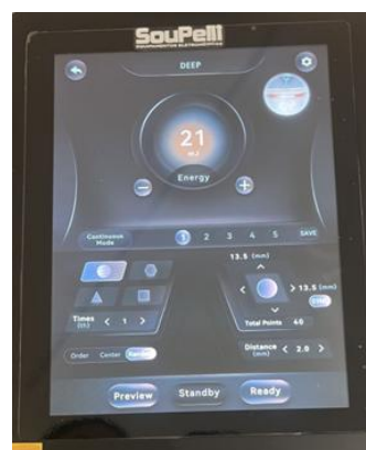
Image 2: Control panel of the fractional CO 2 laser in deep mode showing a point application configuration, demonstrating the operational parameters used in patient 1 with energy of 21 mJ per point, intercolumnar spacing between points of 2.0 mm, and randomized firing pattern. It has 40 points per cycle, allowing precise control of the density and total thermal load applied to the tissue.
