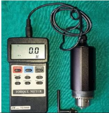
Lutron TQ® -8800 Digital Torque meter for evaluating maximum insertion torque
