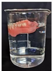
FIG 6- Water test used to ascertain the hollow space which is revealed by the floating denture
