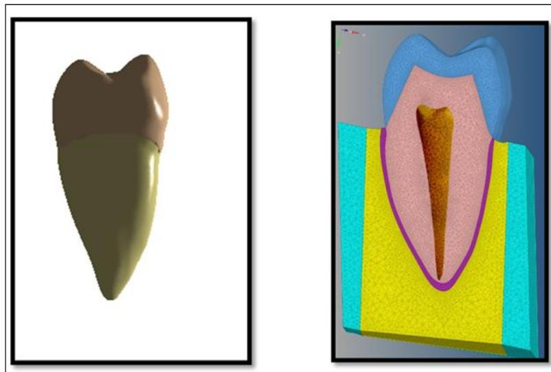
**FIG-4; GEOMETRIC MODEL 1 WITH CORRESPONDING MESH (CROSS SECTION)**
