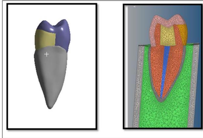
**FIG-3A; GEOMETRIC MODEL 2 WITH CORRESPONDING MESH (CROSS SECTION)**
