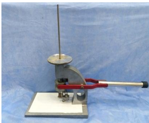
Fig. 1: Showing the portable deadweight device as described by Pachioni et al.
