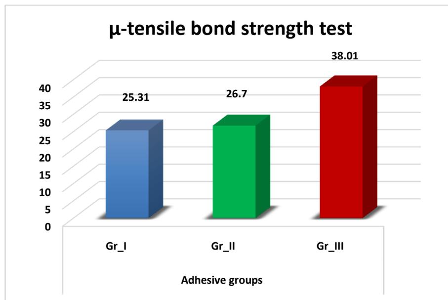
Figure 6: Column chart representing the mean values of  $\mu$ -tensile bond strength between all adhesive groups
