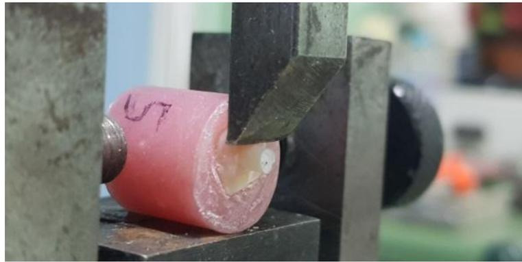
Figure 5: specimen for micro shear bond strength
