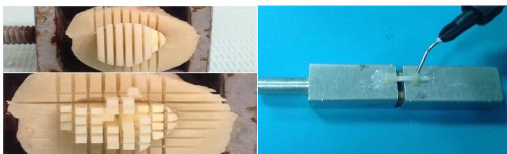
**Figure 4: specimen for micro tensile bond strength**
