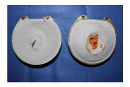
Figure.6. After dewaxing of the pattern
