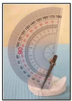
Fig. (3): Simple tool to measure the angle on the model.
