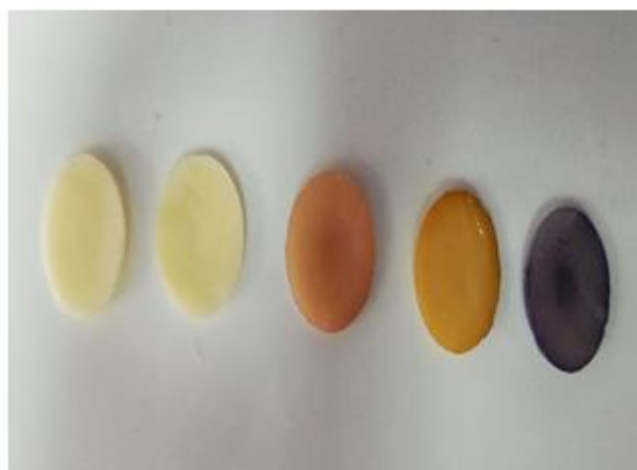
Figure 3. Discs after the test period, left to right: control, coca-cola, wine, coffee, tea.
