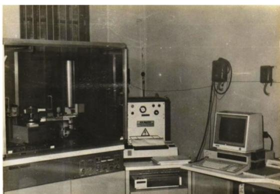
Fig. I: RIGAKU X-RAY DIFFRACTOMETER
