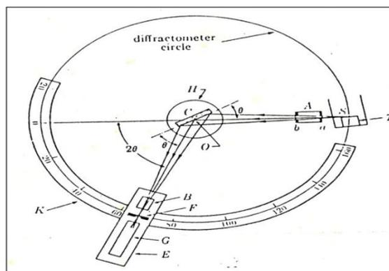
Fig. II: SCHEMATIC WORKING PRINCIPLE OF X-RAY DIFFRACTOMETER
