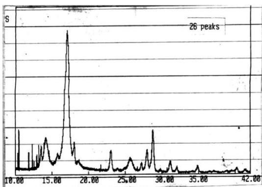
Fig. VII: X-RAY DIFFRACTION PATTERN OF STRUVITE
