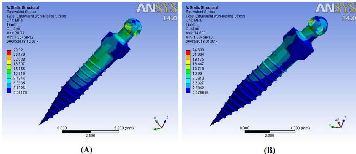
**Figure 4:** Von mises stresses on miniscrew inserted at 60° in bone when C.B.T was 0.5 mm (A), Horizontal force (B), Oblique force.
