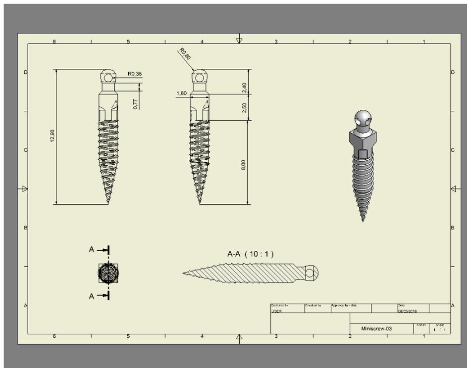
**Figure 1:** Miniscrew design on Autodesk Inventor screen based on manufacturer dimensions.
