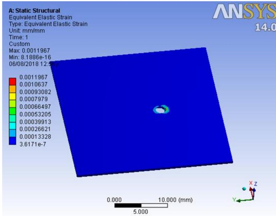
**Figure 6:** Microstrain on cortical bone when horizontal force was applied on 60° inserted miniscrew and C.B.T was 0.5 mm.
