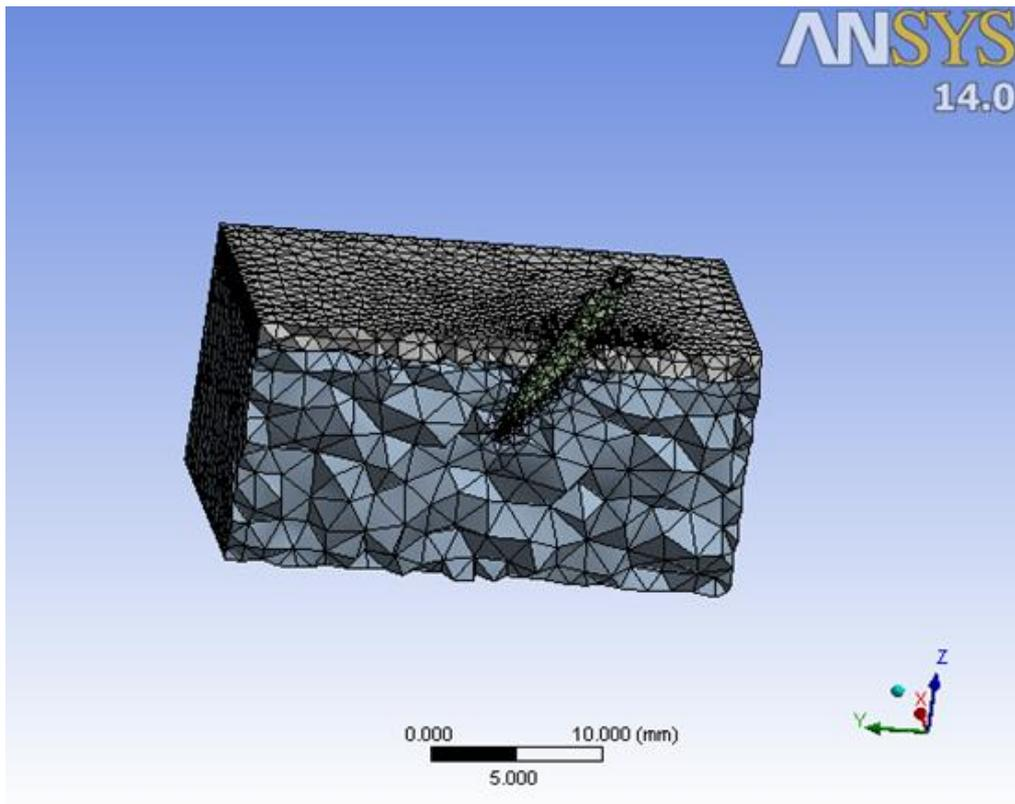
**Figure 2:** Complete longitudinal cut section in 60° inserted miniscrew.
