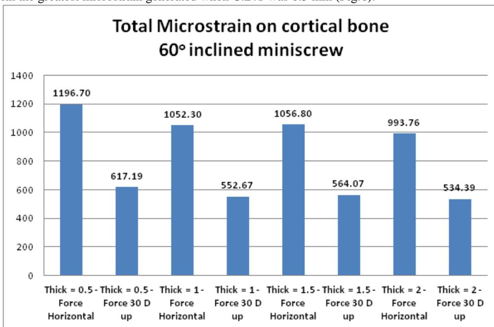
**Figure 5:** Bar chart showing microstrains on cortical bone of different thicknesses when insertion angle was 60° to bone surface and 2 N force applied in two directions.
