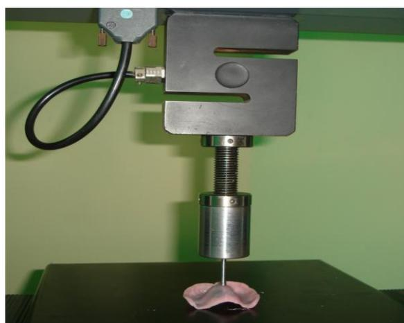
**Fig. 23** Denture bases on UTM
