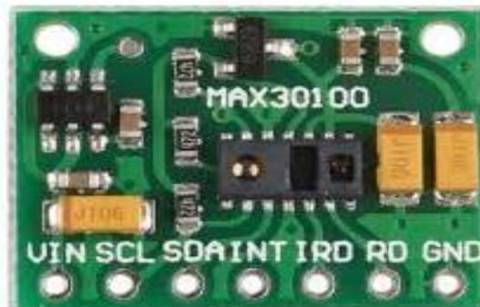
MAX30100 operates on a supply in the range of 1.7 to 2V. It reduces power consumption and visible light emission when the user's finger is not on the sensor. Ultra-low power operation increases battery life for wearable devices. Application of MAX30100 is, fitness assistant devices, medical monitoring devices and wearable devices.
