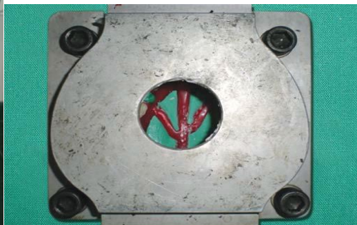
injection moulding flask
