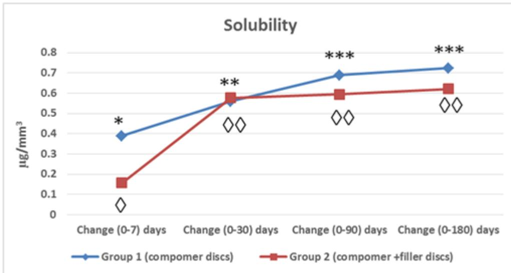
Figure7. Line diagram representing means of solubility change ( $\mu\text{g}/\text{mm}^3$ ) over time of the two groups, \*  $p \leq 0.05$  for group 1,  $^{\diamond} p \leq 0.05$  for group 2. Different symbols indicate statistically significant difference between different time intervals and same symbols indicate statistically non-significant difference.
