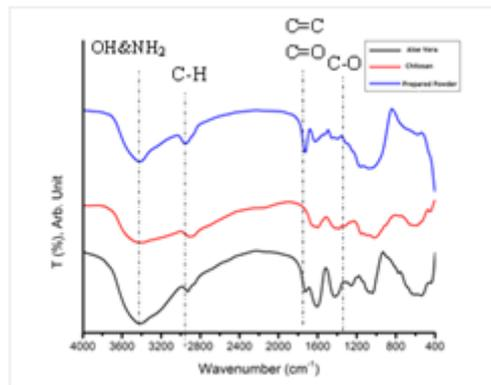
**Figure 2.** FTIR spectra of the asreceived Aloe Vera, chitosan and the prepared powder.
