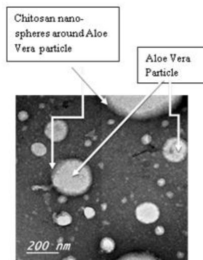
**Figure 4.** TEM micrographs of the prepared powder, where the areas of high electron density represent Aloe Vera and areas with lower electron density represent chitosan
