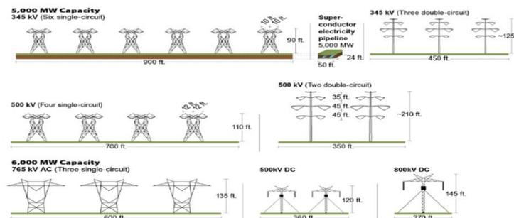
**Fig. different types of tower for transmission line**
