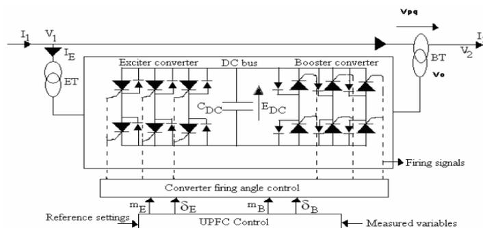
Fig. back-to-back voltage sourced converters.
