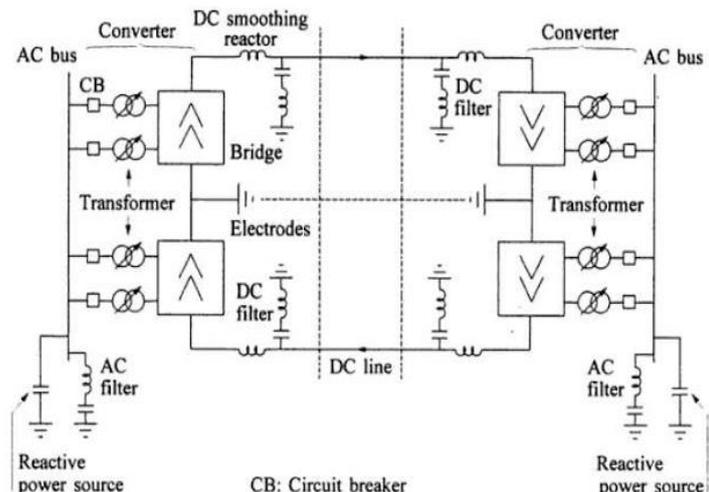
Fig. main components of HVDC system
