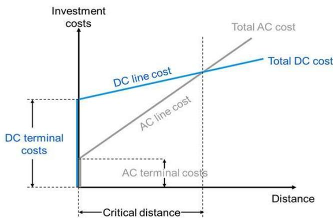
Fig. Cost analysis of AC and DC transmission system
