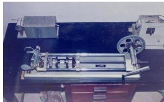
Fig-5-Hounse Field Tensometer
