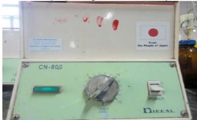
FIGURE 2 Microcapillary centrifuge used in M.C.B.S. technique
