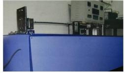
Fig: 4 Reciprocating Sliding Wear Test Machine
