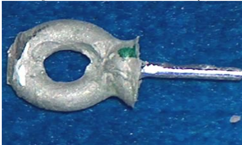
Figure 3: Custom made special device constructed to ensure vertical application of tensile force.
