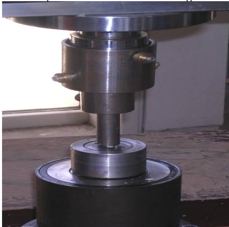
Figure 3: Custom made special device constructed to ensure vertical application of tensile force.
