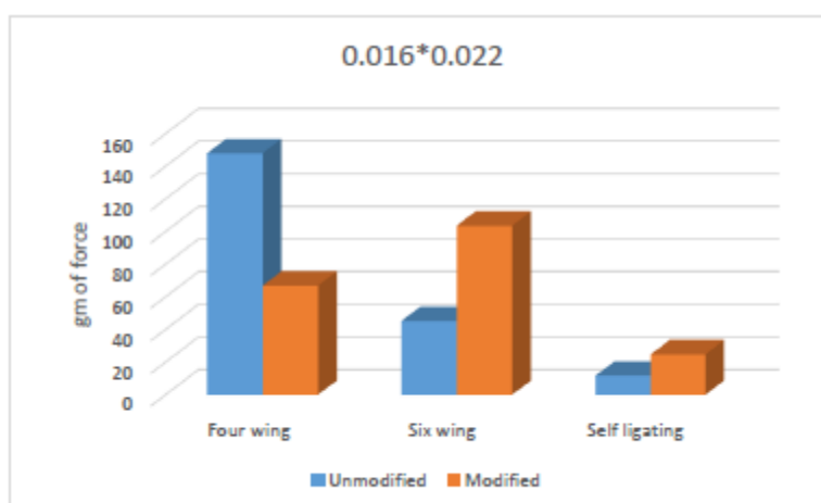
Figure (5): Mean of Static Load of different brackets with 0.016x0.022 Wire.
