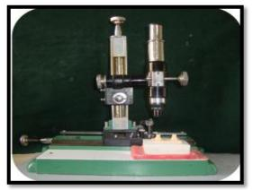
Fig.6 Travelling microscope with cast
