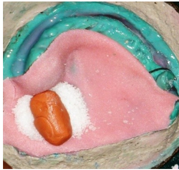
Figure 3: NaCl packed with silicone putty
