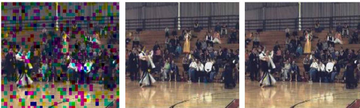
a) Inter P 209 frame with PLR=20%. (b) Inter P 209 frame EC without Intra-frame EC. (c) Inter P 209 frame EC with Intra-frame EC.
