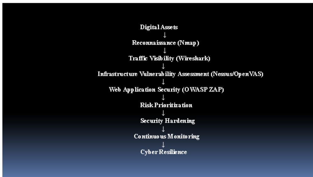
Figure3: Proposed model of Integrated Ethical Hacking Evaluation Framework (IEHEF)
