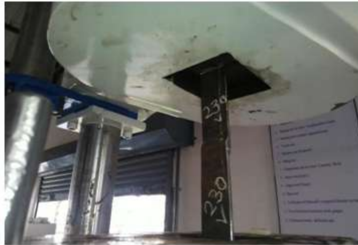
Figure 2 Sample specimen between the holding plates of the UTM during shear test.
