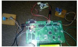
Fig 7 Overall Miners Module Hardware Setup
