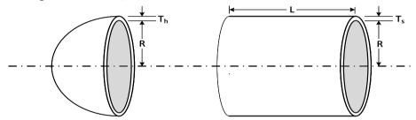
Fig. 2: A pressure vessel
