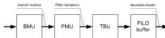
Figure 4: Schematic representation of the Viterbi decoding block
