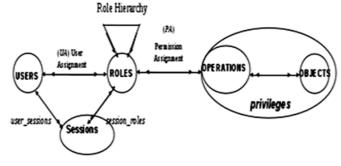
Fig. 2. Role Based Access control Model (RBAC)
