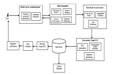
Fig. 1. Security system to prevent information leakage
