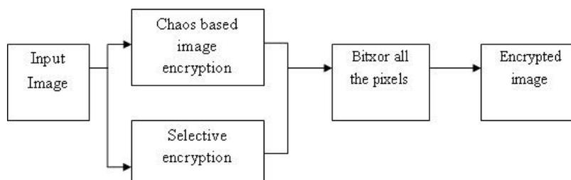
**Figure 4 Proposed Selective Image Encryption technique**
